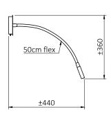
SOURCE: powerled 3w + lens 2700K VOLTAGE: 220-250V POWER: 3W MARKING: CE P2 C WEIGHT: 0,6 kg
